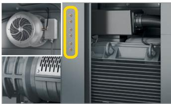
**External grease fitting lubrication**
