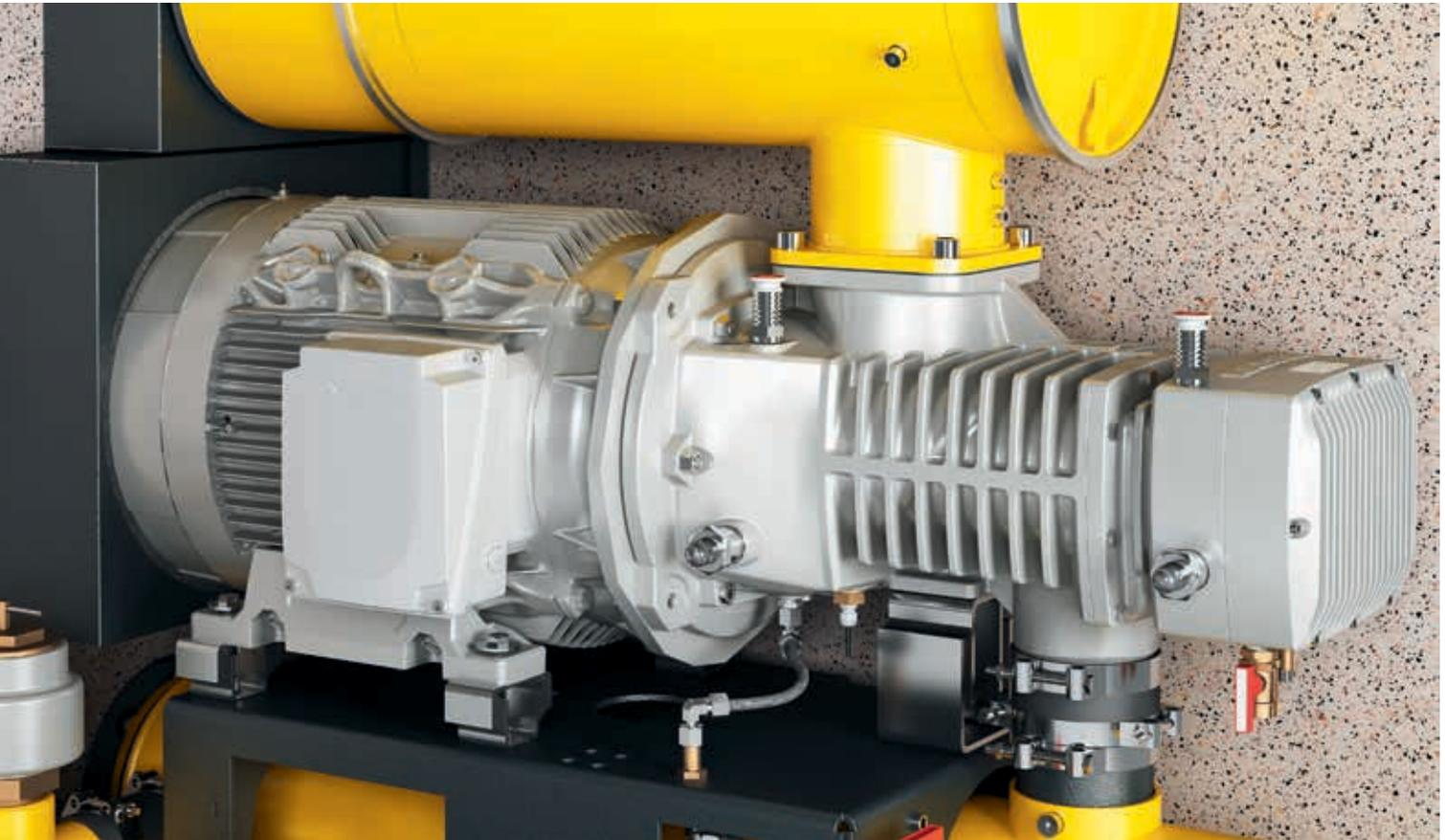
In CBS and DBS series blowers, power is transferred from the motor to the blower air end via an integrated gear drive. Following detailed testing in Kaeser's Research and Development Centers, this was found to be the most effective transmission solution for the speeds in this power size and machine class with regards to efficiency, dependability, and durability.
