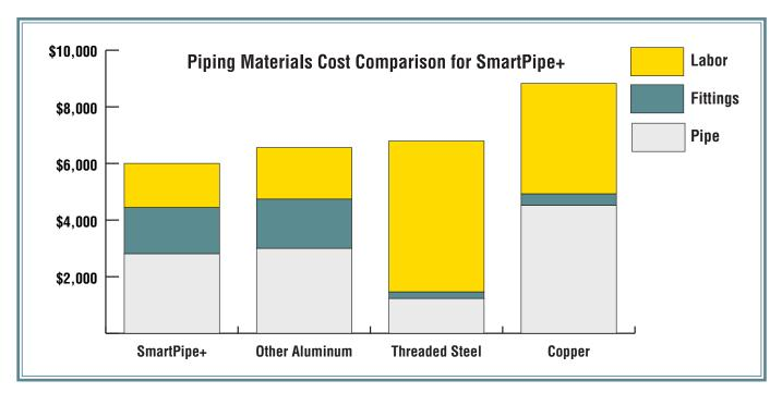
Based on: 500 feet of 2" pipe, sixteen elbows, seven tees, and ten couplings. Labor rates calculated by using MCAA labor with rates factored at 0.70.
